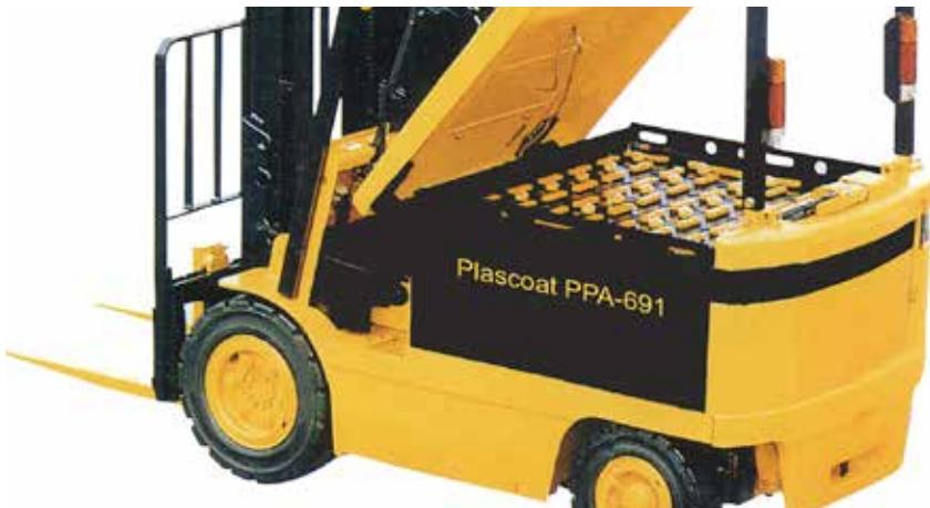
Acid and impact resistant storage systems for batteries are required for vehicles and for essential power back-up systems.
