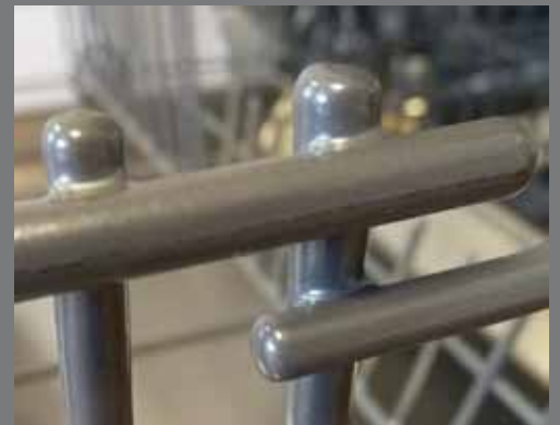
Plascoat Talisman 10 provides comprehensive coverage for complex edges and wirework
