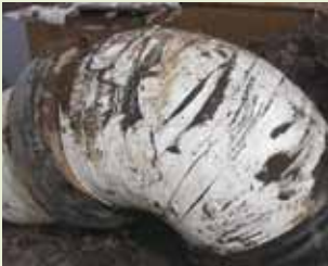
▲ Ductile iron pipe with deteriorated PVC tape wrap after 5 years.
