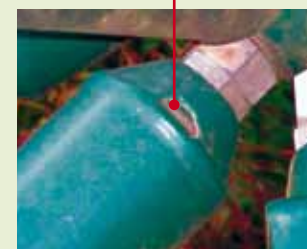
▼ No corrosion under the coating after 12 years
