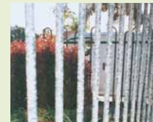
▲ Aluminium fencing coated in green polyester after just 18 months by the sea in Brisbane, Australia.
