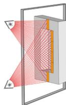
The scanned object contour is translated in several segments in order to position and activate each single gun accordingly.
