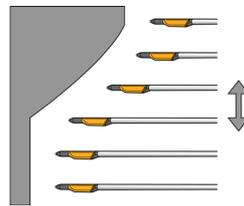
Depending on part geometries the guns may oscillate up and down or remain in a fix position.
