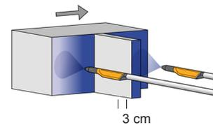
Detection of struts or projections > 3 cm up to line speeds of 5 m/min.
