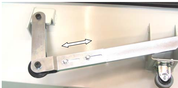
Waste powder container - setting the stroke on the handle
