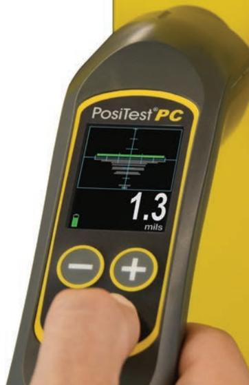
*Target Grid simultaneously displays distance to the part and alignment, making measurements easy*
