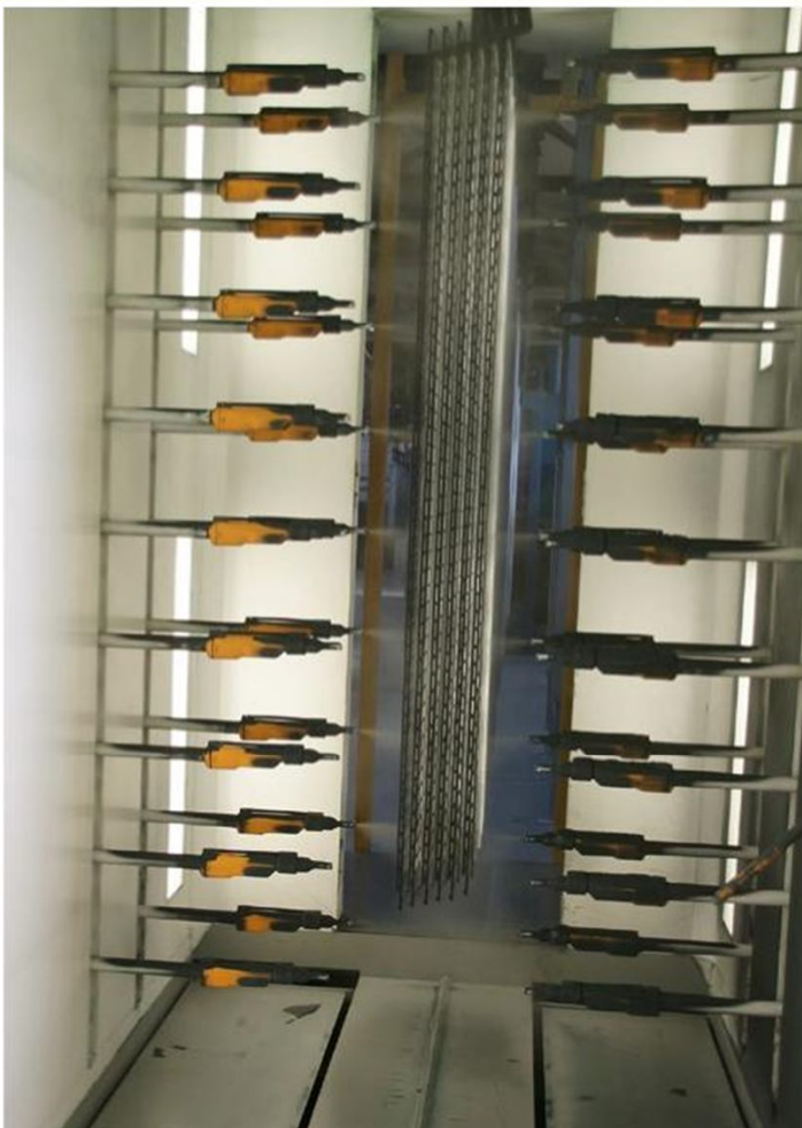
Spray booth is equipped with 36 automatic guns; they ensure ideal paint coverage of open-work elements.
