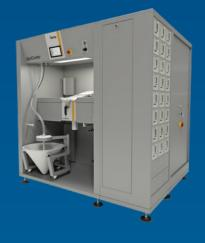
The OptiSpeeder is equipped with an automatic fresh powder supply and a powder-level control system that ensures a constant quantity of powder in the container. The suction pipes for the injectors are considerably shorter than in conventional powder centers. These features translate into an even more uniform powder flow and improved coating results.
