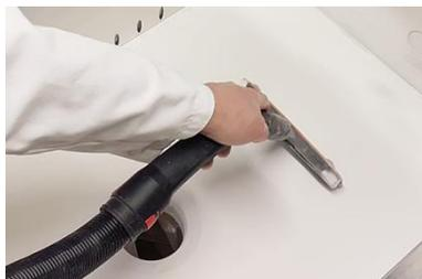
3. Visually check the OptiHopper interior, clean with the suction unit and/or with the compressed air gun if necessary
