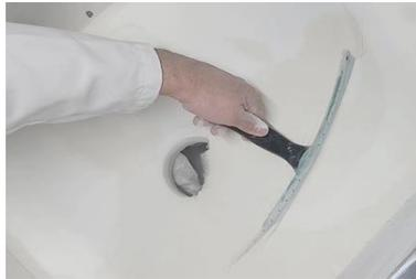
26. Use a scraper to clean the side walls of the OptiHopper so that the suction openings are no longer covered with powder.
