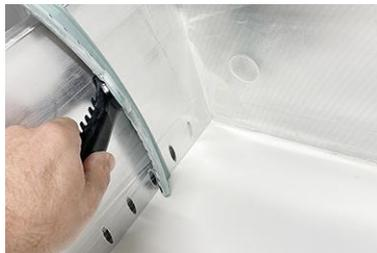
27. Also clean the fluidizing plate so that there is only a small amount of powder on the surface.
