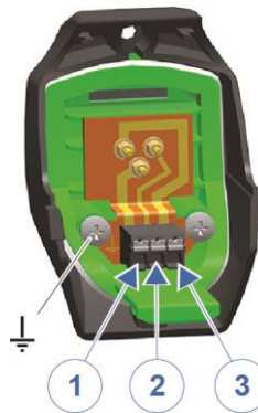
Fig. 13: Lid – Connections (cable numbers)
