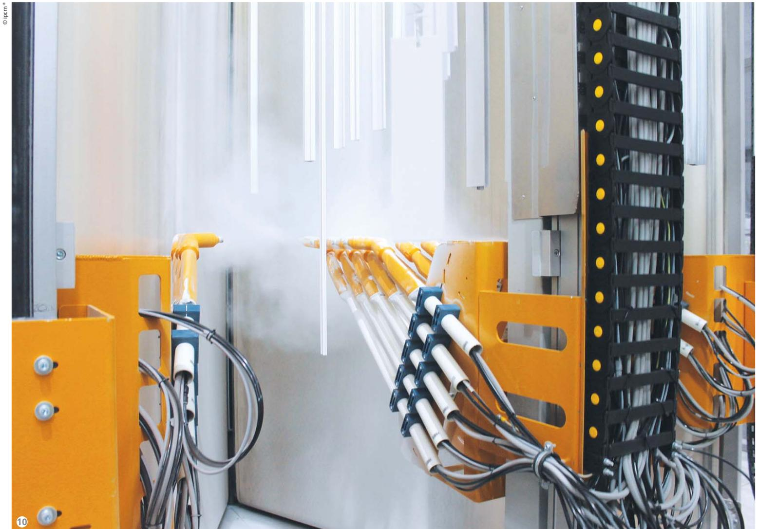
Figure 10: In the V-shaped booths the guns are arranged on both profile sides.
