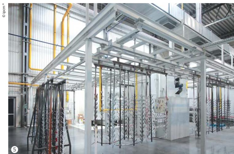
Figure 5: One of the two horizontal painting installation used by Aliplast.
