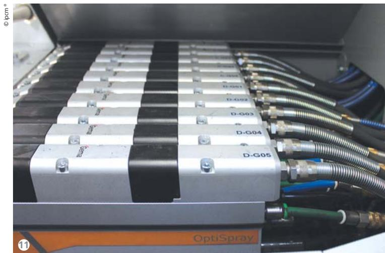
Figure 11: Aliplast Poland's coating booths are equipped with GEMA OptiSpray dense phase pumps.
