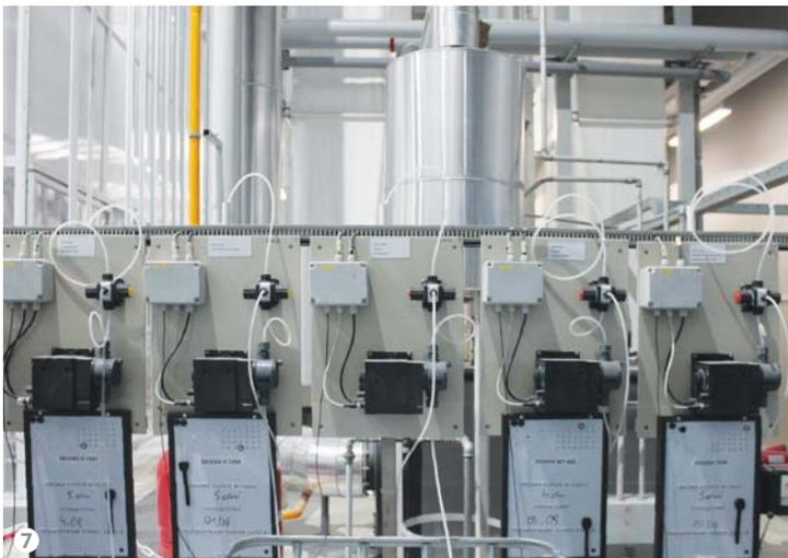
Figure 7: The dosing modules of the pre-treatment tanks of the new vertical installation.
