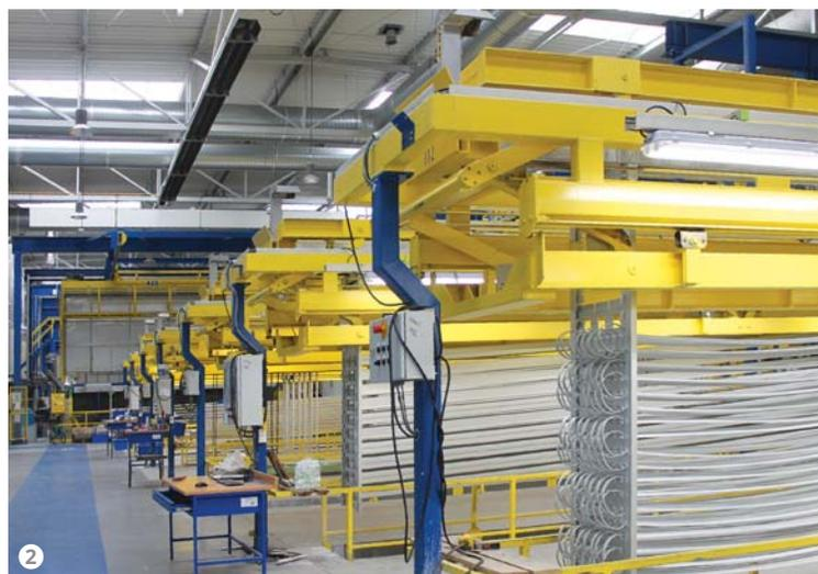
Figure 2: Profiles hung onto the anodising line.
