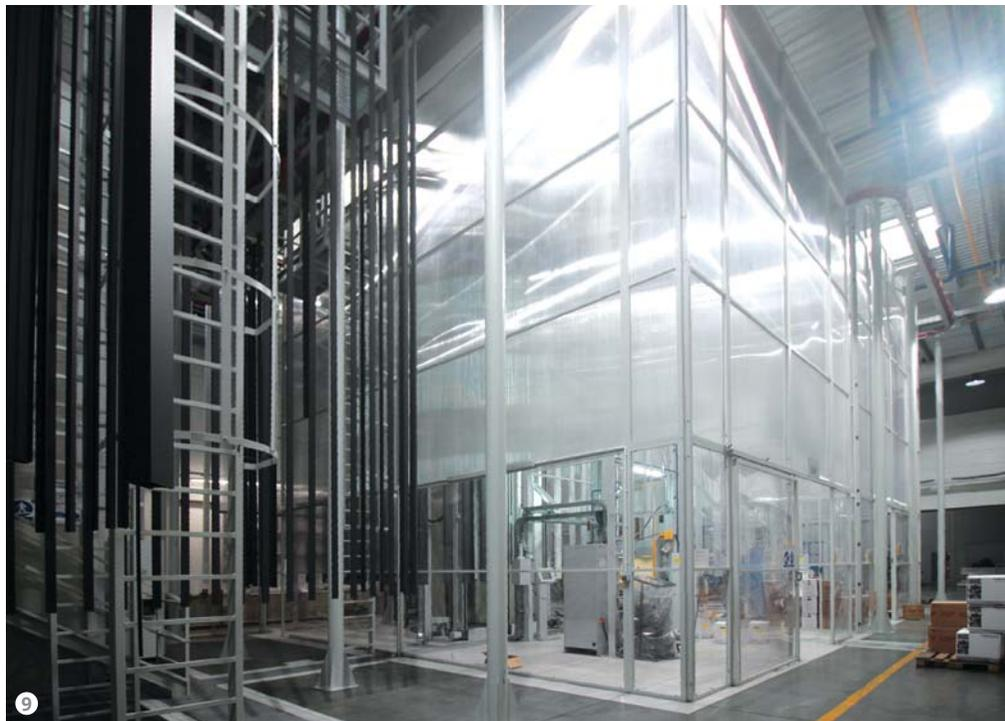
Figure 9: The enclosed area containing the two application booth of the new installation.
