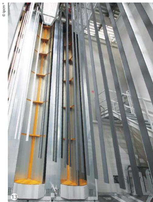
Figure 13: The revolving doors at the entrance and exit of the drying and curing units.
