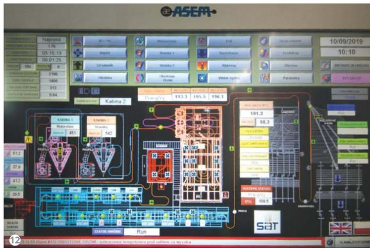
Figure 12: The touch screen for the complete management of the plant.
