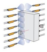
Gap detection Gap detection is the base for the «no part – no spray» function.
