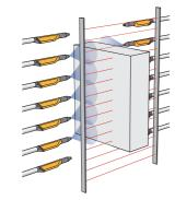
**Height Recognition** Depending on the detected object height only the required guns are triggered.
