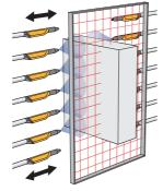
Width Recognition Automatic adjustment of the horizontal gun position according to the object width.
